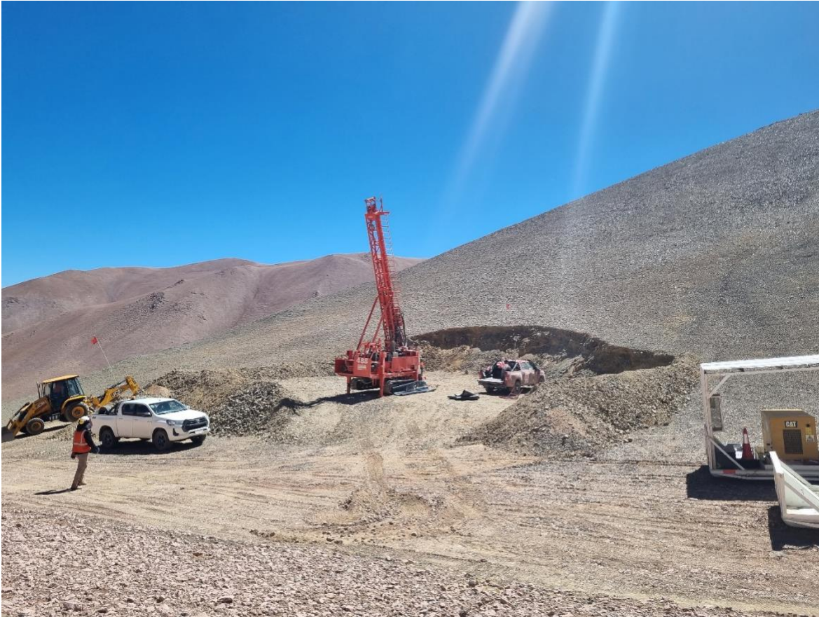
Figure 2. Diamond drill rig positioned for the maiden drill hole at La Peña
